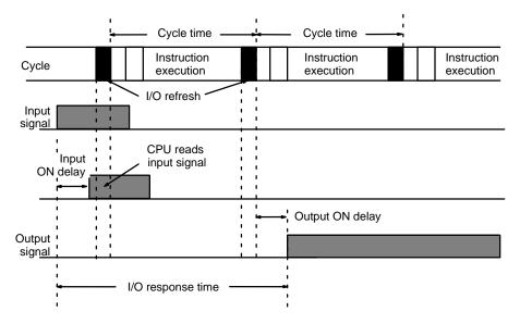
Minimum I/O response time = Input ON delay + Cycle time + I/O refresh time + Output ON delay
